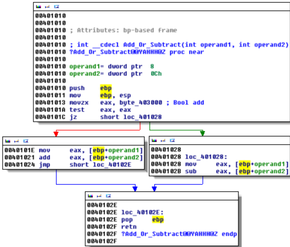
Figure 2: Disassembly of the Add_Or_Subtract() function.
